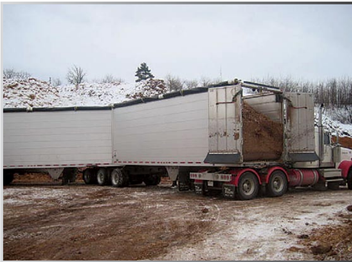
Split loads can be unloaded quickly through the front of the lead trailer by jack-knifing the truck and operating the live floor in reverse.
