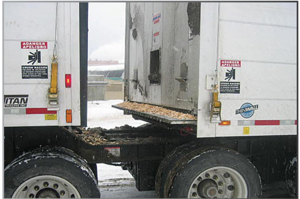
The secret to creating a 62'8" trailer that can self unload is the hydraulic system that pulls the two trailers together.
