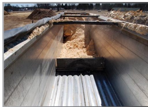
With a custom kicker plate and V-Plow system, Handrich trailers unload cleanly to save time picking up backhauls.
