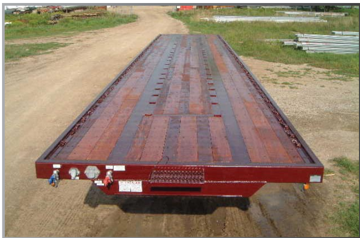
Fabricated steel T's drop into square-cut holes in the deck; a choice of three different T positions allows quick assembly of bunks for fast, stable loading of steel coils.
