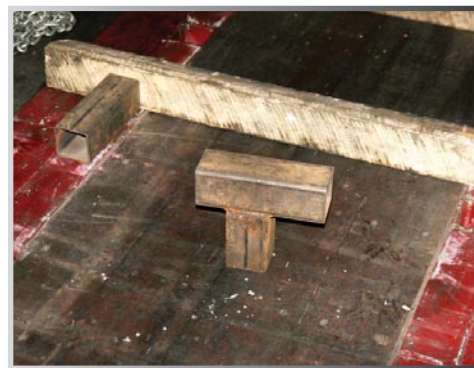
The offset shape of the steel T's provides additional flexibility for positioning the timber bunks.
