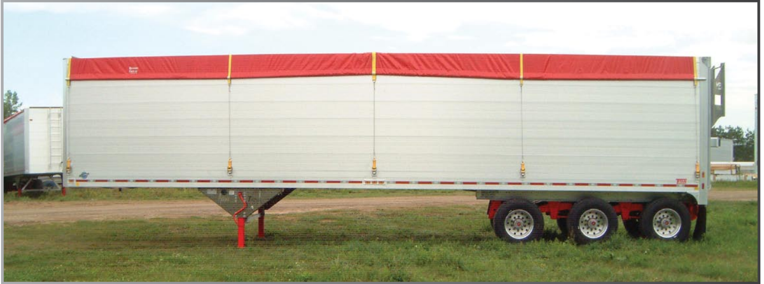
Each unit of the A-Train is sized to suit tipper floors originally built for loading rail cars.
