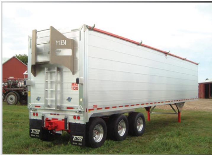
The Rocky Mountain Double was designed in conjunction with MBI to carry 234 cu. yd. of municipal solid waste per truck.
