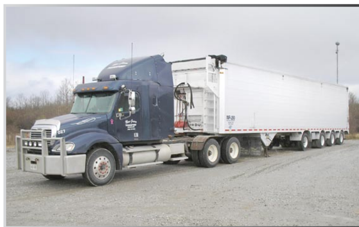
The smooth sides inside and out combine for increased volume and better fuel economy.
